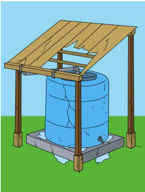
Figure 17: Households should be able to maintain and fix water storage tanks in order to ensure that they are functional at all times. This supports adaptive capacity because it increases available capacity to store water in times of drought.
